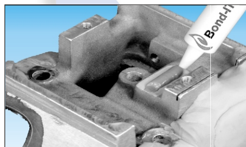
Bond-IT 7056AL Fills a Casting Before Re-Machining
