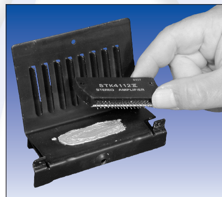
Duralco™ 132 Dissipates Heat in a Semiconductor Device
