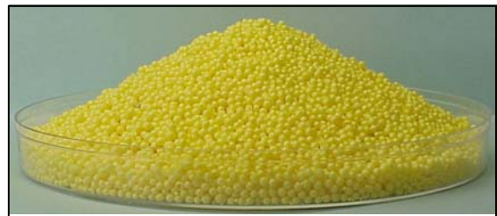
ZHB-1 flows freely to a low 30° angle of repose
